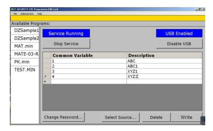
dataZen Engineering's P-SECURITY provides an Okuma P100 II, P200 or P300 control user with the ability to have the associated Part Program automatically retrieved from local or network location, p-selected into the control ready to run, and call an associated setup instruction file.
